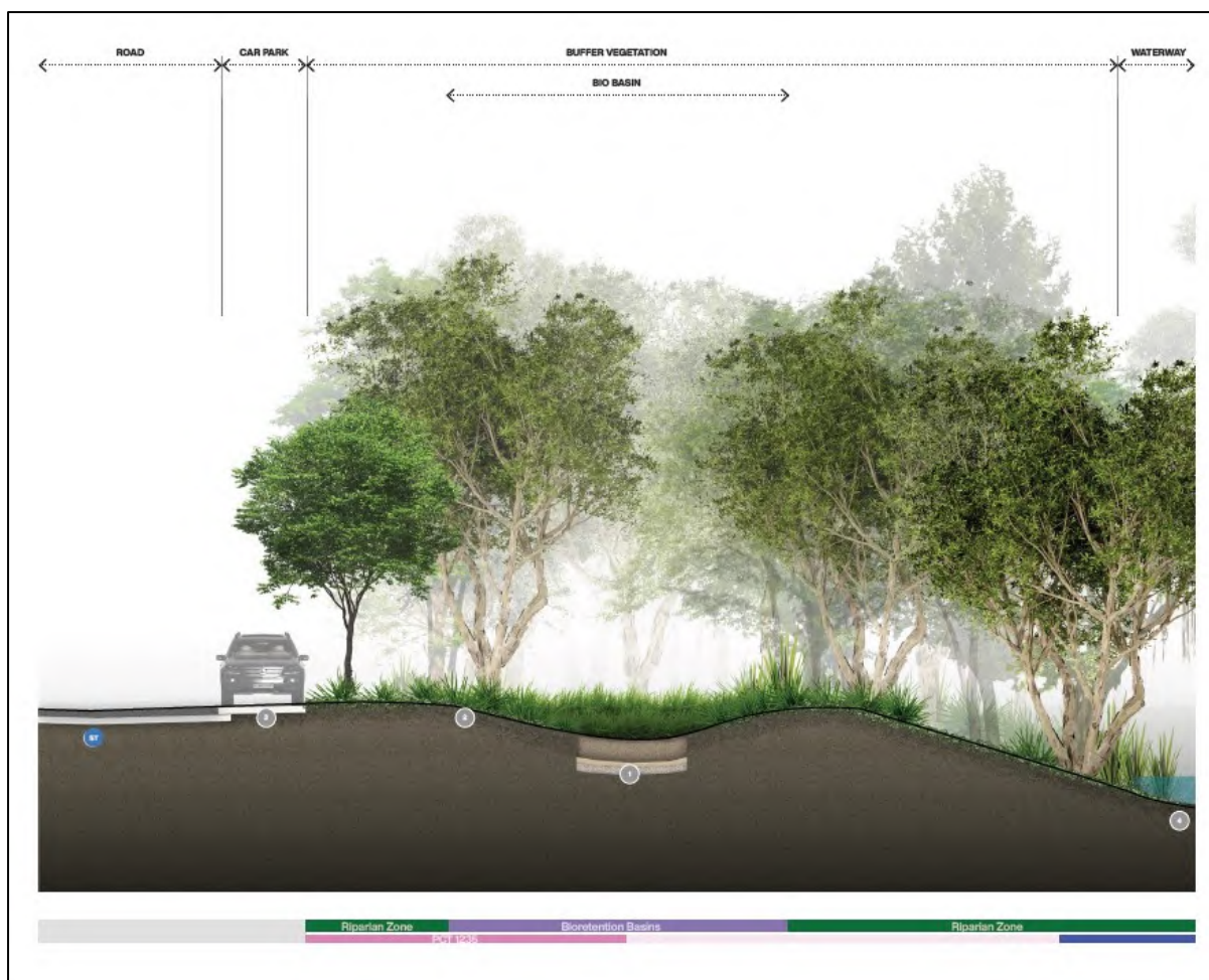
Figure 4 Excerpt from Statement of Landscape depicting an example of integration of stormwater management devices with revegetation zones (Zone Landscape Architecture 2024)
